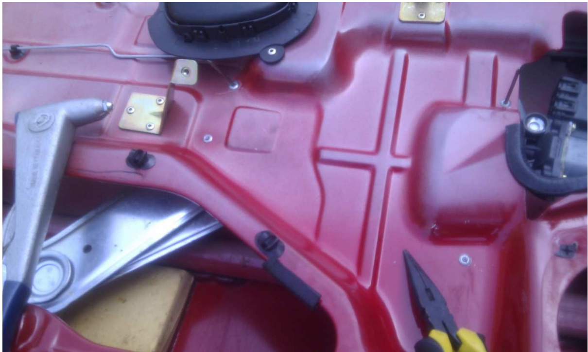
Here I am returning the fixing clip to the window lifter runner track on the new door (cheers Ade).
