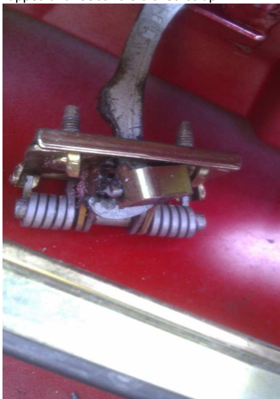
This image is to show the snapped and foobar'd old checkstrap.
