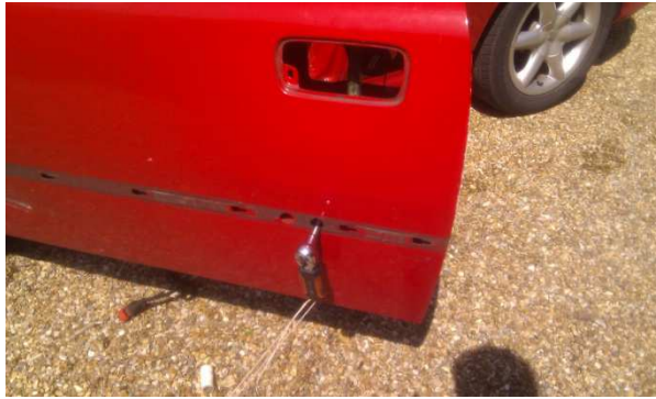
Here I have removed the front glass support bracket, makes removing the glass easier.
