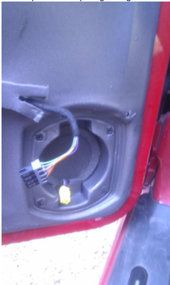
Picture to show speaker void with speaker loom poking through.
